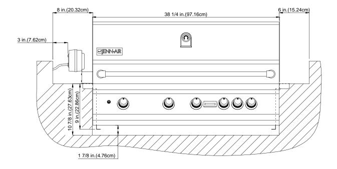
The following are minimum dimensions necessary to install the 4 burner + 1 sear burner built-in grills:
